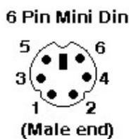
The mouse connector and the keyboard connector on a modern PC have similar pin configurations. Due to this, the keyboard or mouse is not damaged, if plugged into the wrong hole, but it will of course not work as expected. ☺
